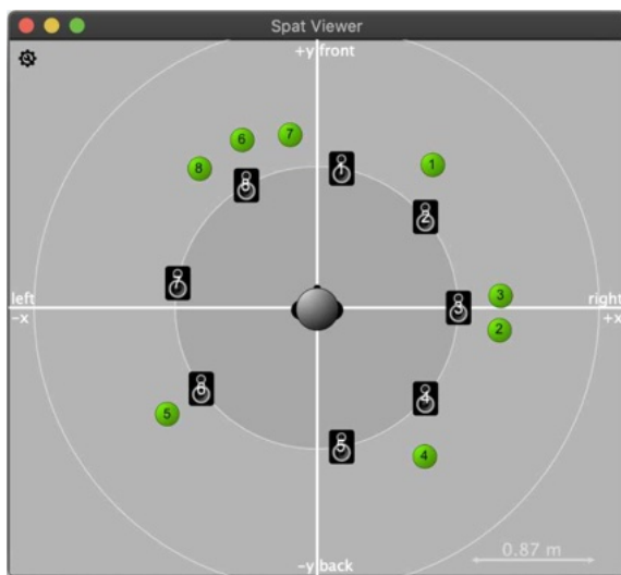
Figure 7: The loudspeaker array configuration of the CIR within the Spat5 Viewer interface. Black boxes represent fixed loudspeakers, while green circles denote movable sound sources.
