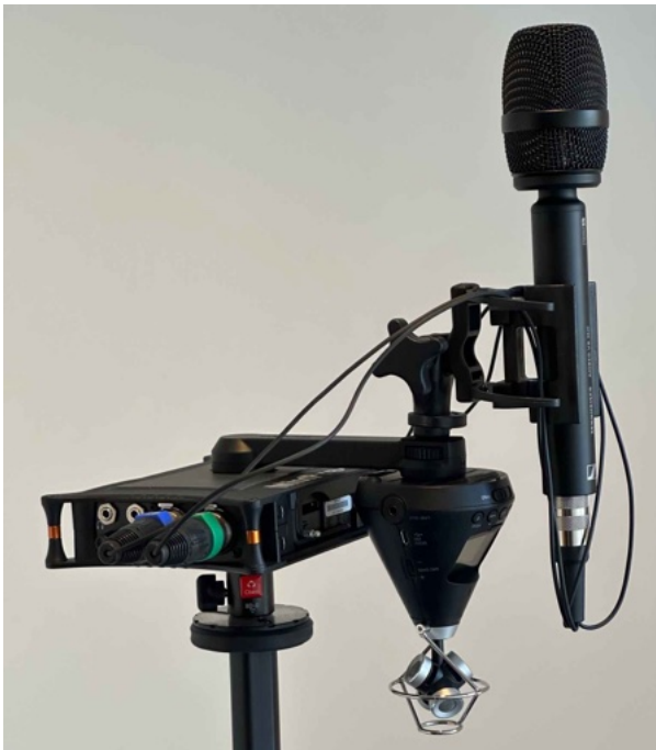
Figure 6: Setup example to ambisonic recordings - H3-VR (Zoom) and Sennheiser (AMBEO) microphones combined with a Mix Pre 6 sound device. This approach offers efficiency and portability, enabling the reproduction of comprehensive spatial audio information with relatively compact equipment. Note that in this image, both microphones were together, but just one is necessary to do the recordings; in this case, we used both to compare the results.
